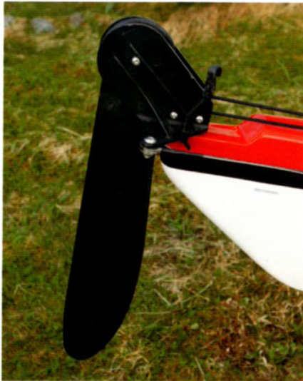
NorthSea has an effective rudder which can be tipped up on deck.
